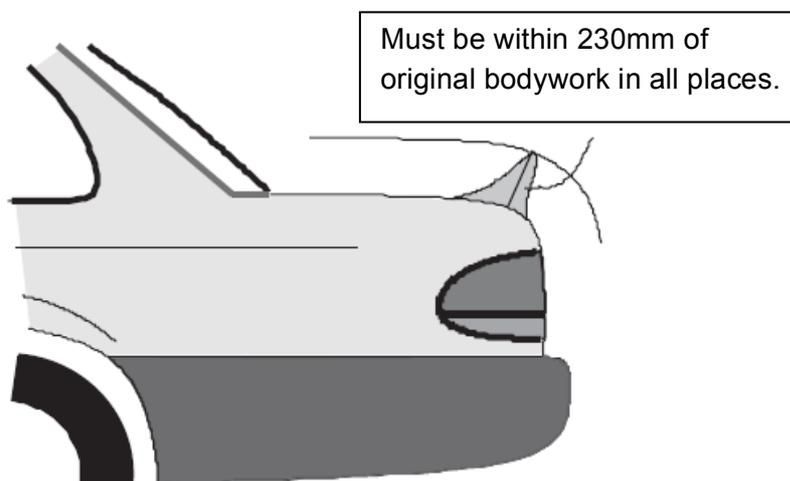
The aero package may be a mix of custom and commercial available packages provided the maximum dimensions of A are adhered to.
